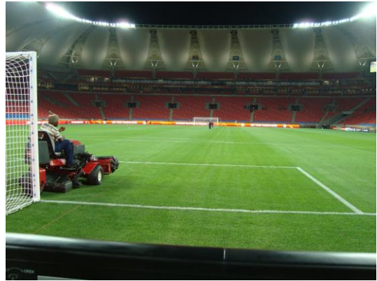
Goals not removed prior to mowing – poor maintenance practice that creates unnecessary wear in the goalmouths.
