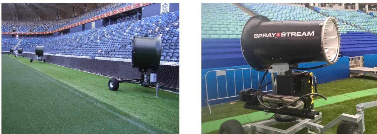
Fig. 11. Examples of pitchside ventilation and cooling fans used to manage turf health.
