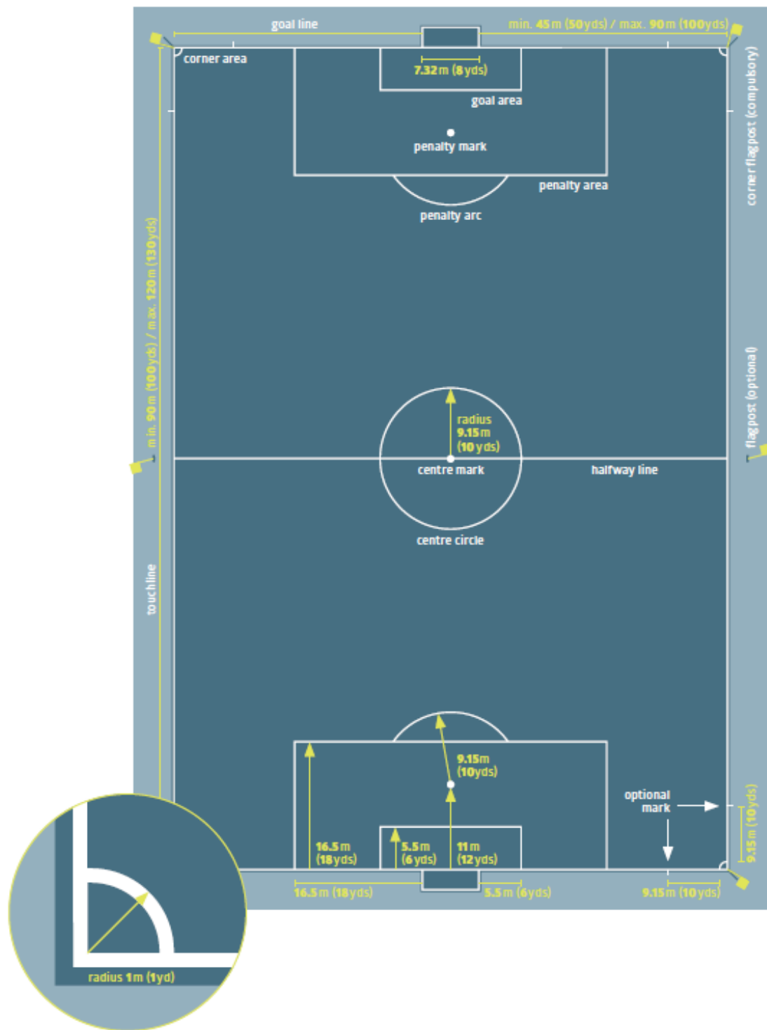
Fig. 17. Overview of pitch dimensions and line marking requirements (source: IFAB). Note: lines are considered part of the areas they delimit. The optional corner dashes marked outside the pitch (9.15m from the outside of the corner areas) should be 24cm long, starting 12cm from the goal line/touchline.
