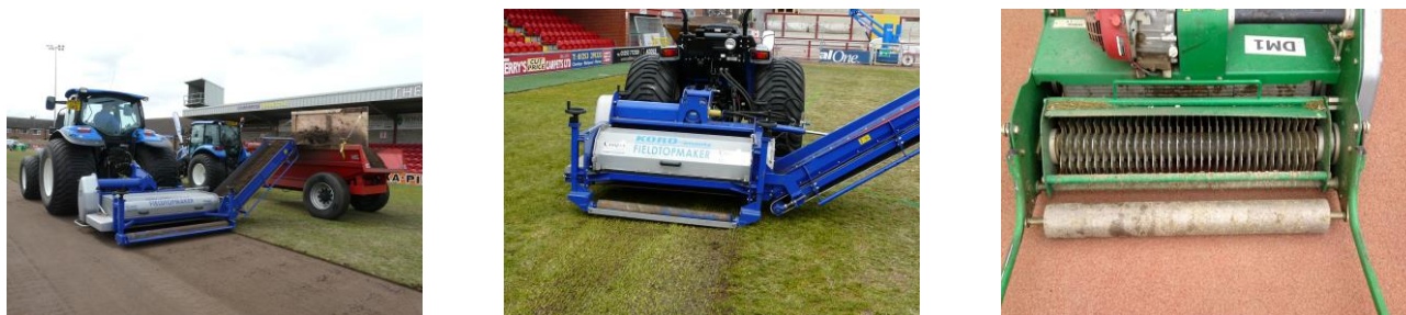
Fig. 23. Different types of thatch control and removal. From left to right: complete surface removal, deep scarification and verti-cutting. All three types have very different aims and objectives.
