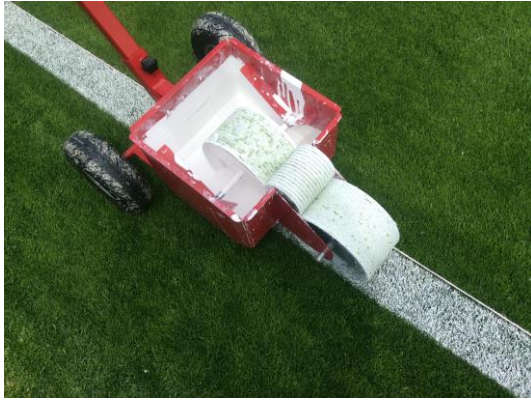
Fig. 18. Wheel-to-wheel line marking following a string line (left) and marking out dashed lines (right).
