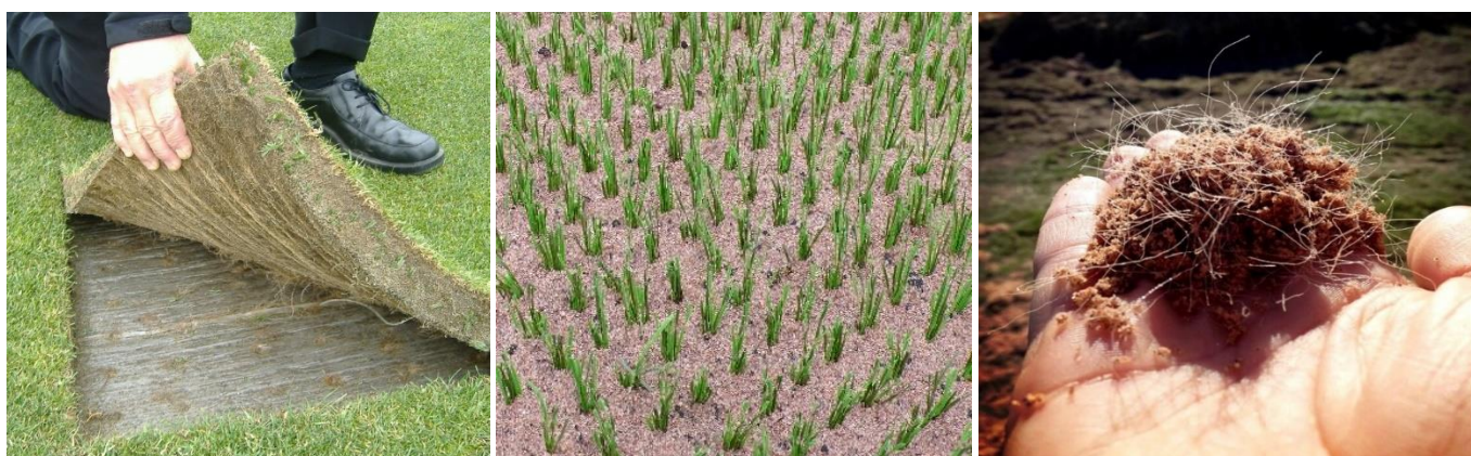
Fig. 5. Types of turf reinforcement system. From left to right: carpet, stitched and fibre.
